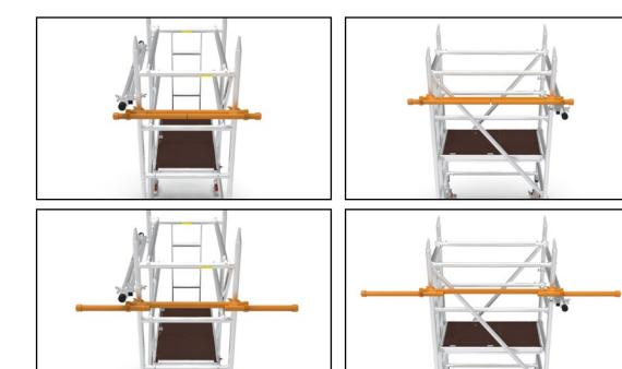
These should be positioned horizontally in the area between the 2 guardrails for the platform (approx. 750m above the platform). There are 2 couplers on each stabiliser that connect to the frame uprights.
